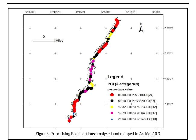
prioritize the sections. This repetitive process to select sections that can be maintained with available budget is done by adjusting the PCI threshold values.
