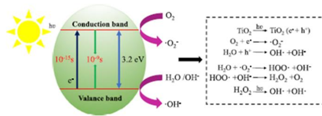
Figure 11. Engineered nanomaterial is the proposed mechanism for the photo catalytic elimination of contamination over TiO 2 ENM (Reproduced with permission from Ref. [68])
