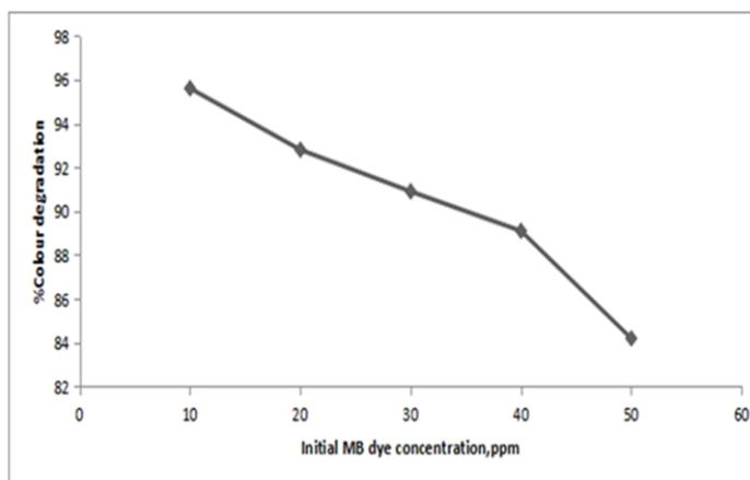
**Figure 5.** Effect of dye concentration on degradation percentage of MB dye. Operating conditions:  $[Fe^{2+}] = 4mM$ ,  $[H_2O_2] = 70mM$ ,  $pH=3$ , reaction time=60mins,  $T=25^{\circ}C$
