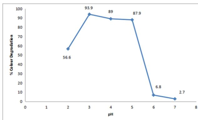
**Figure 1.** Effect of pH on degradation percentage of MB dye. Operating conditions:  $[H_2O_2] = 7.0\text{mM}$ ,  $[Fe^{2+}] = 4\text{mM}$ , reaction time=60mins,  $[MB] = 20\text{ppm}$ ,  $T=25^\circ\text{C}$
