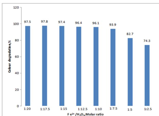
**Figure 4.** Effect of [Fe<sup>2+</sup>]/ [H<sub>2</sub>O<sub>2</sub>] ratio on degradation percentage of MB dye. Operating conditions: pH=3, [Fe<sup>2+</sup>] = 4mM, reaction time=60mins, [MB] =20ppm, T=25°C
