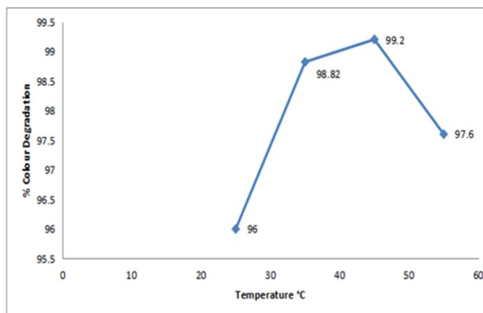
**Figure 6.** Effect of temperature,  $[Fe^{2+}] = 4mM$ ,  $[H_2O_2] = 70mM$ ,  $pH=3$  reaction time=60mins
