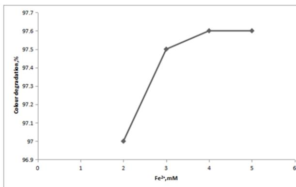
**Figure 3.** Effect of Fe<sup>2+</sup> concentration on degradation percentage of MB dye. Operating conditions: pH=3, [H<sub>2</sub>O<sub>2</sub>] = 70mM, reaction time=60mins, [MB] =20ppm, T=25°C
