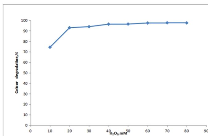
**Figure 2.** Effect of  $H_2O_2$  dose on degradation percentage of MB dye. Operating conditions:  $pH=3$ ,  $[Fe^{2+}] = 4\text{mM}$ , reaction time=60mins,  $[MB] = 20\text{ppm}$ ,  $T=25^\circ\text{C}$
