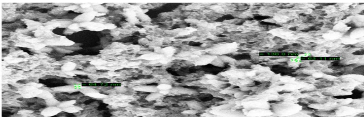
**Figure 3.** The Scanning Electron Microscopy (SEM) of synthesised AgNPs
